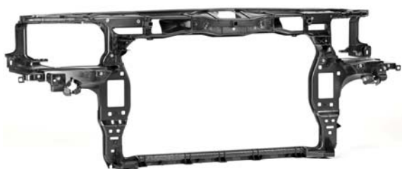
Fig. 1 The lower beam of the front end features an U-shaped profile made of nylon composite sheet.
