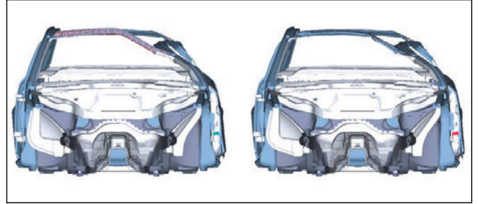
Fig. 13: Results of the roof crush loading case [7]
