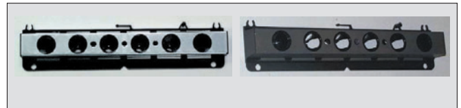
Fig. 6: Test pieces made of galvanized sheet metal (left) and coated with Granocoat (right)
