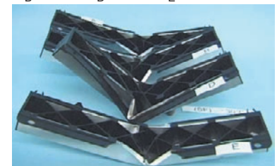
Fig. 8: Results following drop tests with Erlangen carrier [6]
