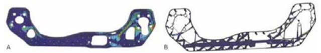
Figure 4 Using finite element analysis (FEA) in the development of the front end (A); in this way, weak points in the metal structure can be detected and optimized at an early stage (B).
