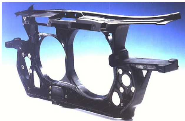
Figure 1 The Audi A6 front end is a hybrid construction, comprising a composite of metal and glass fiber reinforced, elastomer-modified polyamide 6.
