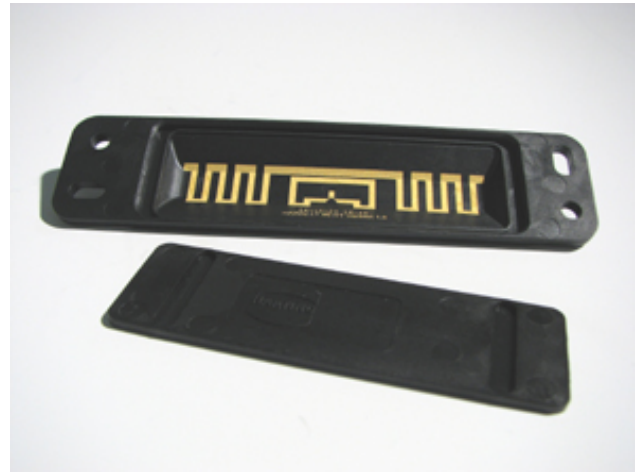
Figure 3 Three-dimensional antenna structure produced using LDS technology
